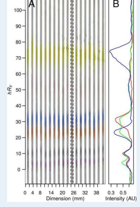
Fig. 4 Chromatograms of the channeled pattern (A) and videodensitogram (B, marked track, in ascending  $hR_F$ : Oracet Violet 2R, Solvent Blue 22, Sudan Red G, Solvent Blue 35, Oracet Red G and Dimethyl Yellow)
