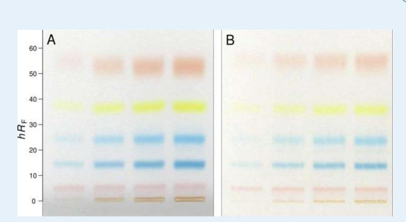
Fig. 8 Comparison of (A) spray-on application and (B) printing of a dye mixture (in ascending  $hR_F$ : E126, E142, E131, E105 and E122) separated on HPTLC plate silica gel 60 with EtOAc - MeOH - H<sub>2</sub>O - AcOH, 65:23:11:1 [7]
