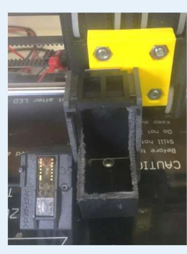
Fig. 6 Sample application via cartridge and holder
