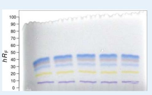
Fig. 9 Printing of both dye mixture (in ascending  $hR_F$ : E151, E110, E132\*, E124 and E132) and mobile phase (MeOH - 5 % Na<sub>2</sub>SO<sub>4</sub>, 3:4 [8]) on HPTLC plate RP-18 W
